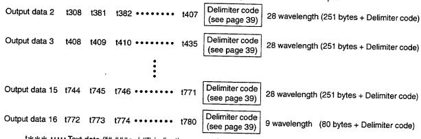
In case of no error, commands and data are transferred between the CS-1000 and personal computer as shown below.
