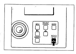
No integration time will be displayed if AUTO, INT.SYNC or EXT.SYNC measurement mode has been selected. To display the integration time, press the SELECT/CANCEL key at the end of measurement.
