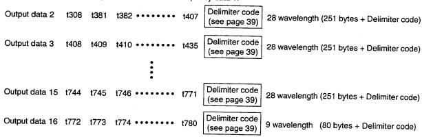
t\*\*\* ..... Text data ("#.###e+/-#") indicating spectral radiance data of the wavelength
